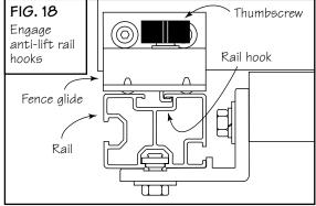
**NOTE:** When removing the TS III from your table saw, always disengage the rail hooks from the T-slot lip before lifting the TS III off the rails.
