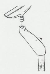
10. Also in 1960, they separated the tool rest arm (503751 - Ref. 167) and the tool rest tube (501354 - Ref. 168) and added a set screw. If replacements are necessary, the (501354) tool rest tube, the (503751) tool rest arm and the (102585 and 102582) set screws should be ordered.
