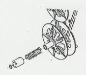
6. In late 1973, starting with Mark V serial #SS3191, the spring case (501657) was replaced with a heavy flat washer and a new, better spring was substituted. The method of holding them on the shaft (retaining ring 501645) is the same. Therefore, if either the old spring cap or the old style spring is ordered, both the new spring (509226) and washer (504553) will be substituted as a pair.
