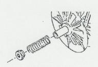
5. Also in 1955, the nut (2802) to retain the sheaves and spring was replaced by a retaining cap and snap ring. The (2895) sheave was replaced with one having a longer bearing/insert. If you have this model, the proper part numbers (above) must be ordered. If owners having this model require a replacement motor, it will be necessary to also purchase a snap ring (501645), a spring retaining washer (504553), a spring (509226) and a floating sheave (504208).
