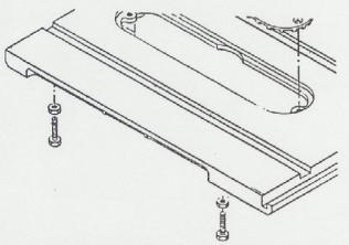
8. In 1960, several minor changes were made in the saw table. When replacing the old table, order assembly (504245) which includes the new table (504246) and front guide bar (501378). They replaced the regular cap screws with nylok cap screws (504252) which eliminates the need for the jam nuts illustrated here.
