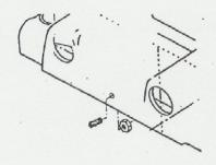
9. At this time they also dropped the 5/16-18 x 1/2" hex head bolt (6327) and the 5/16-18 jam nut (1409) from the carriage and replaced them with a stop ring which rides on the tubeway. The nut and bolt are standard items and can be purchased locally if replacements are necessary.
