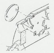
4. In 1955, a 3" hole was put in the back of the headstock behind the name plate. If the old name plate is lost, the new one (504241) will have a spring assembled to it which will have to be removed for your use.
