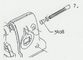
In 1959, a nylon cap (3408) was added to the end of the 202100 drive sleeve assembly. This was primarily a noise suppressor and did not materially change the mechanical operations. This looks like the nylon drive (501295) on the new parts list but it is not the same part. At this time, they also enlarge the hole in the headstock behind the speed control dial.
