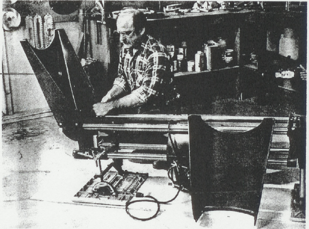
Figure 1. Turn the Mark V over so that it rests on the extension table and worktable, as shown. Then remove the legs.
