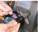
2. Use the 5/32" Allen Wrench to loosen the setscrew in the new Hub Adapter. Slip the Hub Adapter over the Quill Feed Shaft. Align this setscrew with one of the recesses on the end of the Pinion Shaft and tighten the setscrew securely with the 5/32" Allen Wrench, refer to Figure 2.
