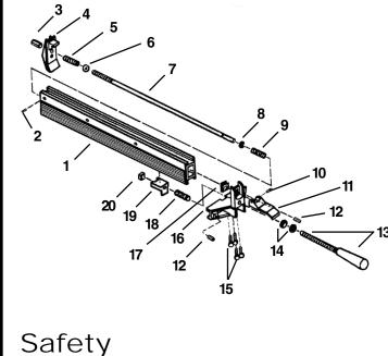
This updates your MARK V Model 500 manual's Parts List and Exploded View for the rip fence, as well as the fence's assembly and alignment instructions.
