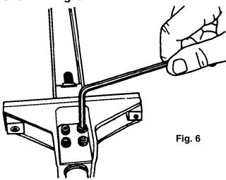
6. Also use a 5/32" Allen wrench to back out both setscrews (12) located in the fence base, as seen in Fig. 7. The setscrews should be recessed into the fence base just enough so they will not touch the fence bar when the fence is attached to the table.
