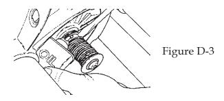
7. When you've lubricated both sheaves, replace the nameplate and the belt cover. Plug in the Mark V and turn it on. Run the machine completely through the speed range several times to help spread the oil out over the shaft and to distribute grease throughout bearings.
