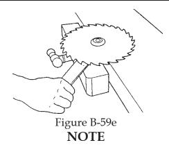
The only time the saw blade is used without the upper or lower saw guards is during alignment and only after the Mark V is turned off and unplugged.
