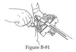
**c.** Return the miter gauge to the slot and recheck and re-adjust it, if needed.
