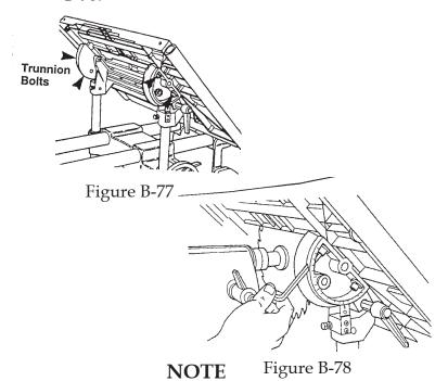
If you find it difficult to loosen the bolts, consider using a T-handle Allen wrench, or use a boxed wrench for extra torque. Another alternative is to use the hanging hole in an adjustable wrench, as demonstrated in Figure B-78a.
