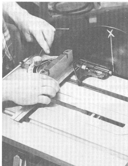
Figure 15. Adjusting the protractor face.
