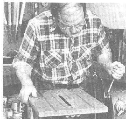
Figure 12. Checking the miter gauge slots.
