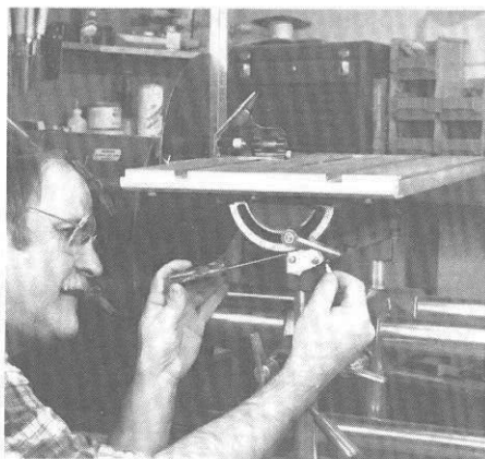
Figure 9. Adjusting the '0' stop.
